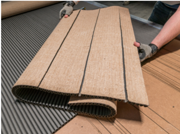
Step 2: Add relief cuts at required intervals.
