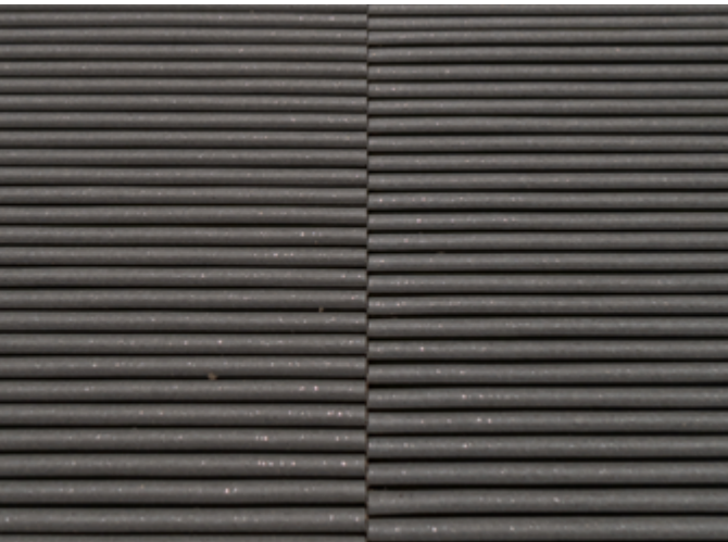
Before: Imperfect rib alignment.
