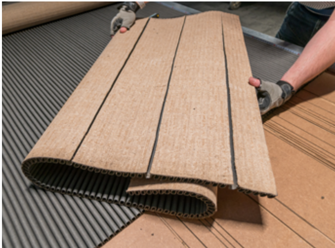
Step 2: Add relief cuts at required intervals.
