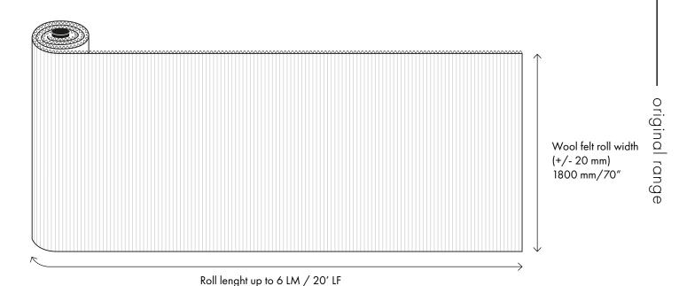
The roll length is to the customer's requirements, with a maximum roll length of approximately 6 linear meters. Ribs run vertically along the roll.
